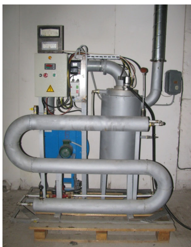
Fig. 2. Photo of a cylindrical immersion heater demonstrator
