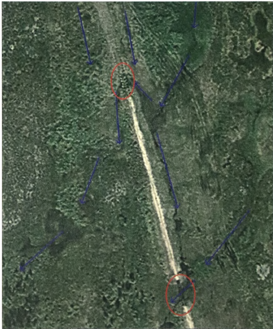
Figure 1. The sector of changing the types of gas pipeline: the underground (at the top) and ground (middle part). The arrows indicate the direction of flow, red colour indicates zones of water discharge through MG
